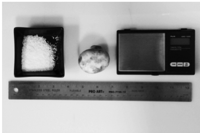
Fig. 3. Materials required for calculating the diffusion coefficient using a mushroom-water system. Clockwise from top left: kosher salt, mushroom, jewelry scale, and ruler.
